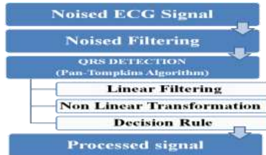
Fig.6. Algorithm flowchart for ECG signal processing
