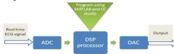
Fig.3. General ECG processing diagram with TMS320C6713 DSK
